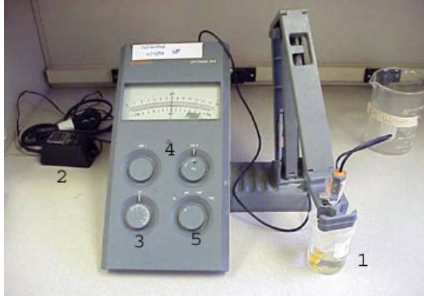
Electrode is stored in storage solution
